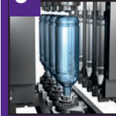
Stretch Blow Molding with hot air
