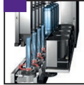
Preform temperature stabilization
